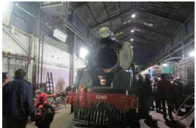
*Lower photo, Mainline Steam's fully operational Ja 1240, with the smoke box door open, undergoing its annual boiler survey. Photos: T.Phillips*
