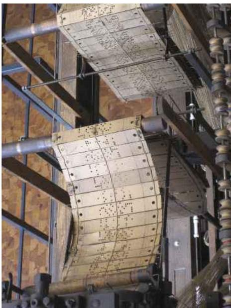
loom produced ribbons of different patterns as determined by the punched cards, as opposed to the Jacquard loom at MOTAT which is a carpet loom. Also in the foyer was a large workable street organ, a working striking clock mechanism and the Cessna 172 airplane suspended overhead in which the young German pilot Mathias Rust flew to Moscow and landed in Red square in May 1987.
