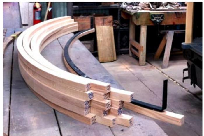
*The curved roof bows for trailer 21 after their delivery from the specialist wood benders Woodform Limited of Henderson. Made from ash, as per the original specifications, the bows are seen here being matched to the previously restored steel framing. Fifteen in total, the bows have since received seven coats of clear varnish and are ready for installation. Problems with the bending procedure meant they had to be laminated instead of being made from one-piece wood.*
