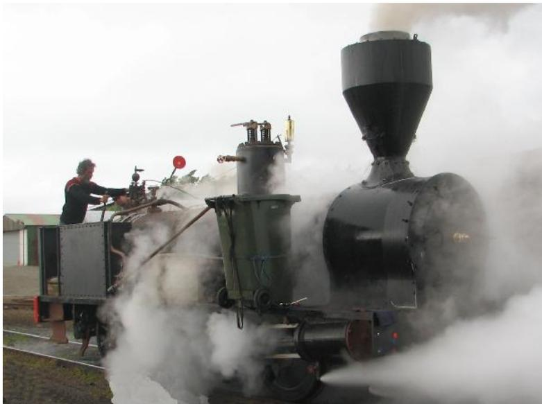
Major items in F180's restoration have included a new front tube plate and steam dome fitted to the boiler, full overhaul of the underframe, new coal bunkers, smokebox and cab rear, and a new steam dome cover. All new parts have been made using the traditional methods including hot-riveting so the loco will be as authentic as possible.
