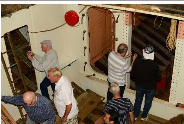
*Inside Toroa's engine room - 99% new steel, with bulkheads that will be watertight*
