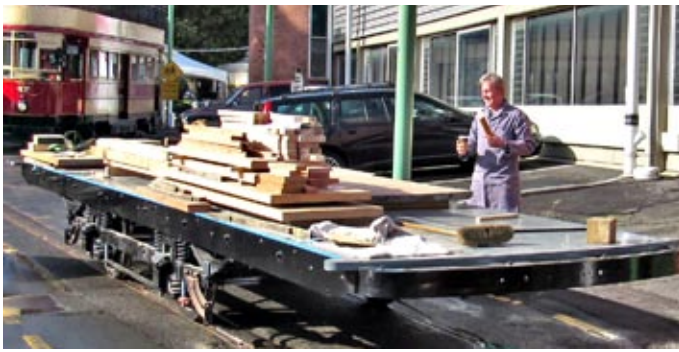
The underframe of 21 rolls out into the sun for the first time on July 24 after the frame was united with the truck. Some of the timber for the body sits on the underframe.
