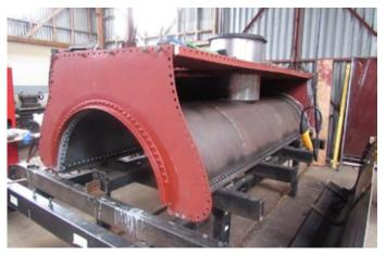
The distinctive saddle water tanks of F.180 Meg Merillees are taking shape in the Rail Section workshops. One side is nearing completion while the sheet metal for the other side has been rolled to shape and is ready to be hoisted and hot rivetted into place. The cylindrical shape on the top of the tanks is for the steam dome.
