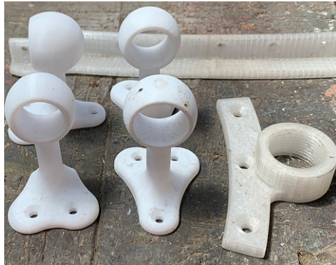
3D printed masters for handrails knobs and bases for trailer 21.
