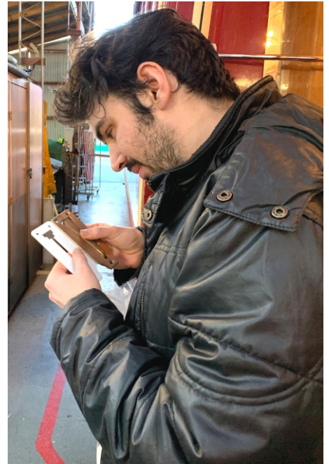
ABOVE: Joseph Dickson inspects a 3D printed latch for trailer 21 against an original.
