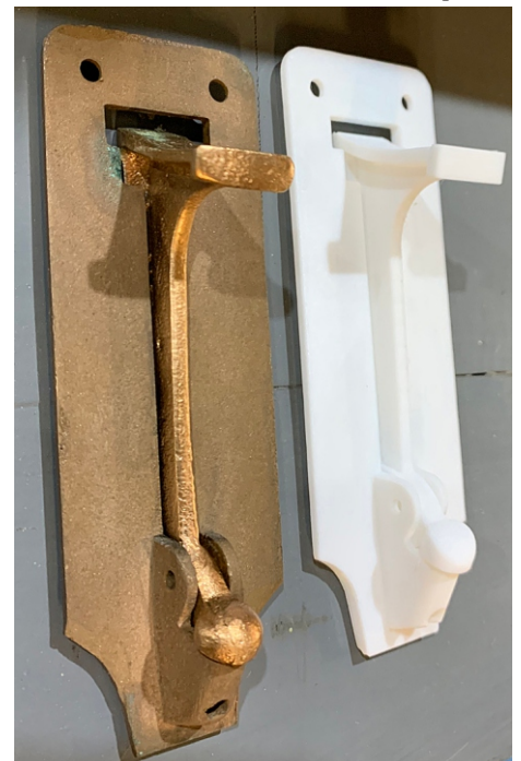
BELOW: The brass original, the only one available, and the 3D printed master for its replacement. Eight will be required for trailer 21.
