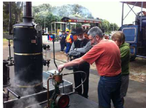
Auckland Steam Engine Society's mobile steam boiler with attached engine
