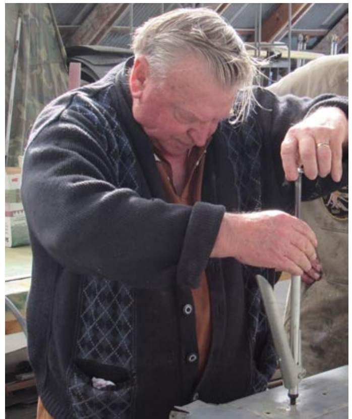
Frank Hannay rivetting the skin on an aircraft panel under restoration at MOTAT.
