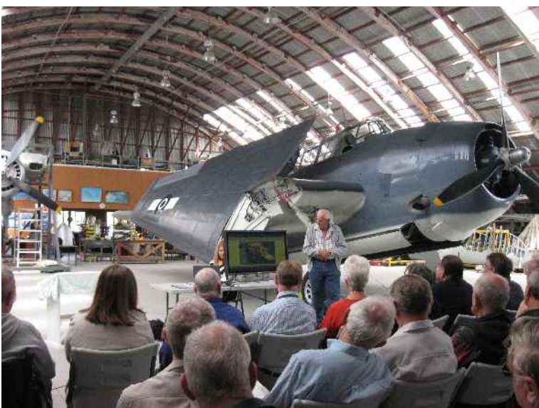
Some of the eighty attendees at the Avenger Launch showing a forward view of the aircraft with the wings in "fold" position, with Norm McKelvey speaking in the foreground. The Avenger was the biggest single engine aircraft of that era weighing eight point one tons A.U.W. This was made possible by the Wright Cyclone R-2600-20 twin bank radial engine with 1900 HP available at take off RPM.
