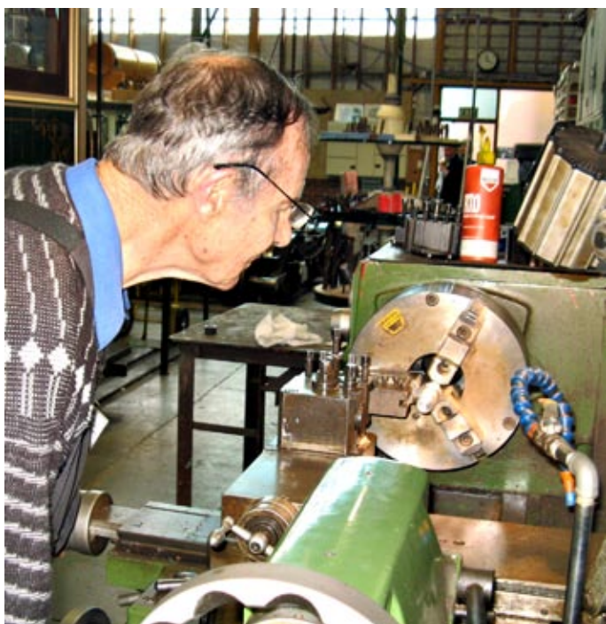
ABOVE: Tony Messenger turning the thread on the one of the eight rods that will tie in the chassis of trailer 21 to the frame that will hold the body in place.
