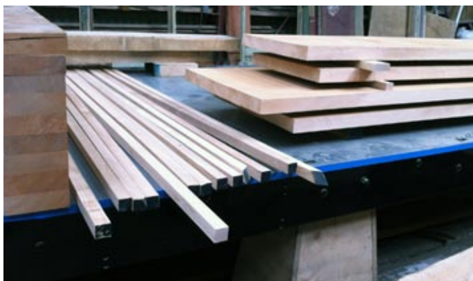
Dressed timber awaiting the next stage of its conversion into timber for the body frame of 21. Left is totara for the roof trusses, centre is ash for the roof bows and right is the kauri for the false roof droppers.
