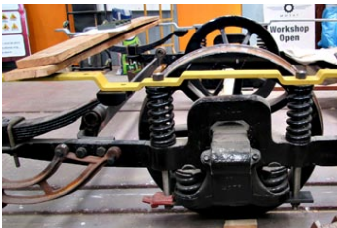
BELOW: The rods in place on one of wheels, running through the springs that will provide the suspension for the body. The yellow coloured body support frame was made from bar steel to the original Brill specifications at Stevenson's East Tamaki workshop.
