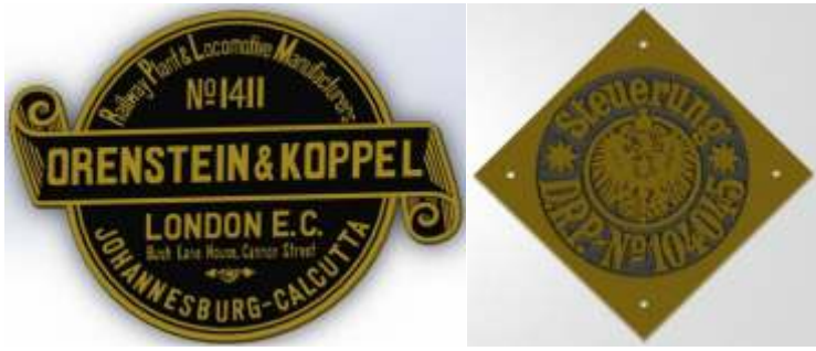
Above: The finished 3D drawings ready for printing. More visible now is the shape in the middle of the patent plate. It is the imperial eagle of Germany. In 1904 Germany was still an empire with a Kaiser on the throne. Patents were issued from the imperial court. Steuerung translates to valvegear with D.R.P. standing for Deutsches Reichspatent, or German Imperial Patent.
