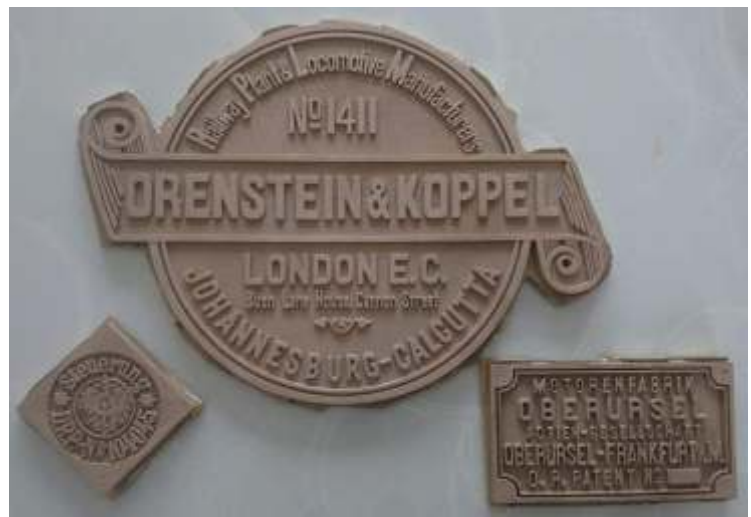
Above: A red letter day - the raw castings after arriving from the foundry.
