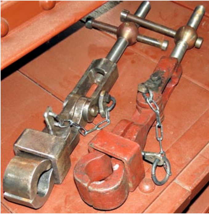
A new rail clamp made by Rail Section members (left) alongside an original which was used as a pattern.
