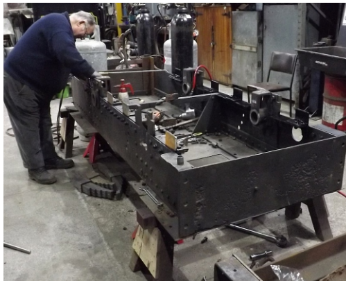
ABOVE: Jim Savage working on the axle boxes on the upturned chassis of the Oberursel. Its sister German locomotive, Bertha, watches on from behind. Photo credit: Richard Croker.
