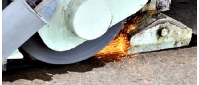
Sparks fly from the grinding wheel as it dresses the track surface, cooled by water from tanks on the roof of the vehicle. The large grey cylinder on the left houses a light for night operation.
