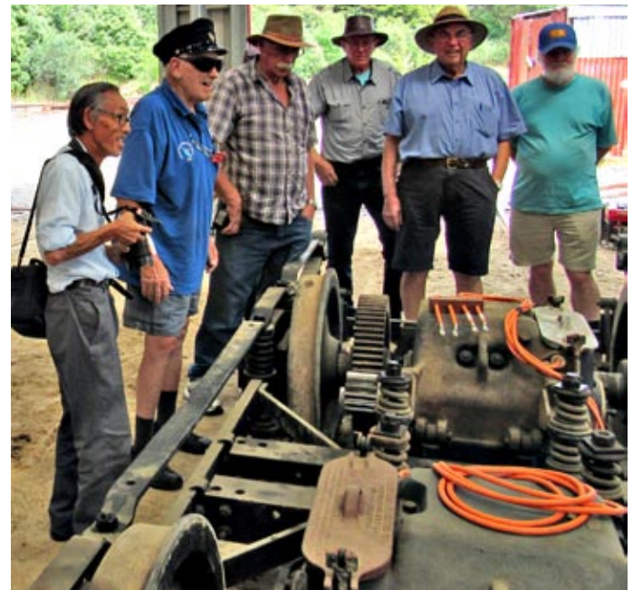
MOTAT Tram Section members inspect a truck for a former Brussels tram at the Whangarei Settlers Museum during a visit earlier this year. The truck will be re-gauged to 3ft 6in gauge to fit the museum's NZR track gauge, and it is planned for the tram to tow a generator on a trailer for power supply. From left they are Albert Chan, Ian Mison, JohnWolf, Bruce Pullar, Chris Cameron and Dave Lennard.
