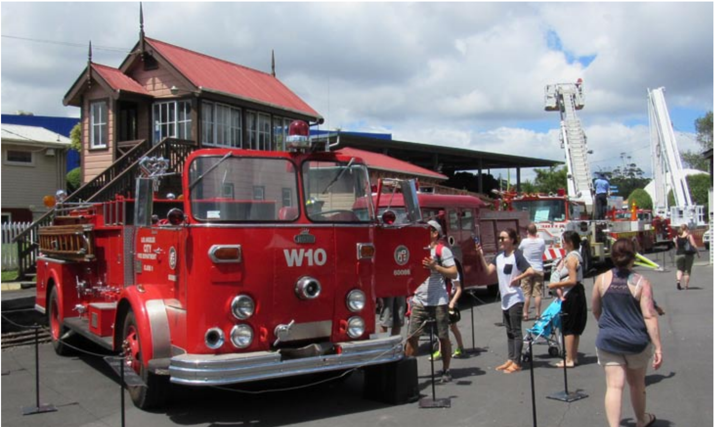
A feature fire truck on display was the Los Angeles City Fire Department's Wagon 10, a Crown Firecoach built in 1961, serial number F1259. W10 is powered by a Hall-Scott 1091 cubic inch petrol engine and fitted with a 1250 gpm Waterous pump and a 400 gallon water tank. After being restored in the US, W10 was donated to the Museum of Transport and Technology in Auckland. Crown Coach Corporation, a school bus manufacturer, made fire appliances from 1951 until 1985, with the Los Angeles Fire Department buying 146 of them. The company became part of General Electric and ceased to exist in October 1990 when its school bus market dried up.
