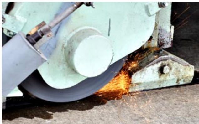
Sparks fly from the grinding wheel as it dresses the track surface, cooled by water from tanks on the roof of the vehicle. The large grey cylinder on the left houses a light for night operation.
