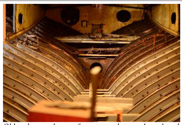
Old and new - the new frames march towards each end of the hull
