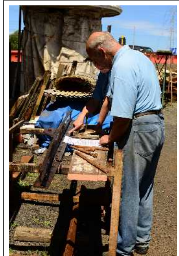
Toroa Society President Don Henwood explains how bad the frames and steelwork was with an example taken from the hull
