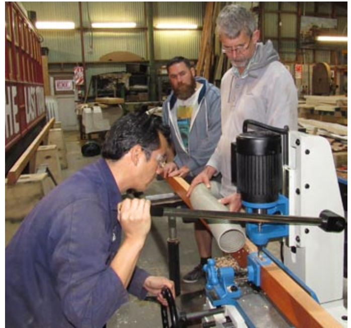
Leyton Chan using a box chisel morticer to cut mortices in the cant rail of trailer 21 for the side pillars to eventually slot into. He is helped by Stephen Curham, holding a vacuum hose, and Charles Richards.
