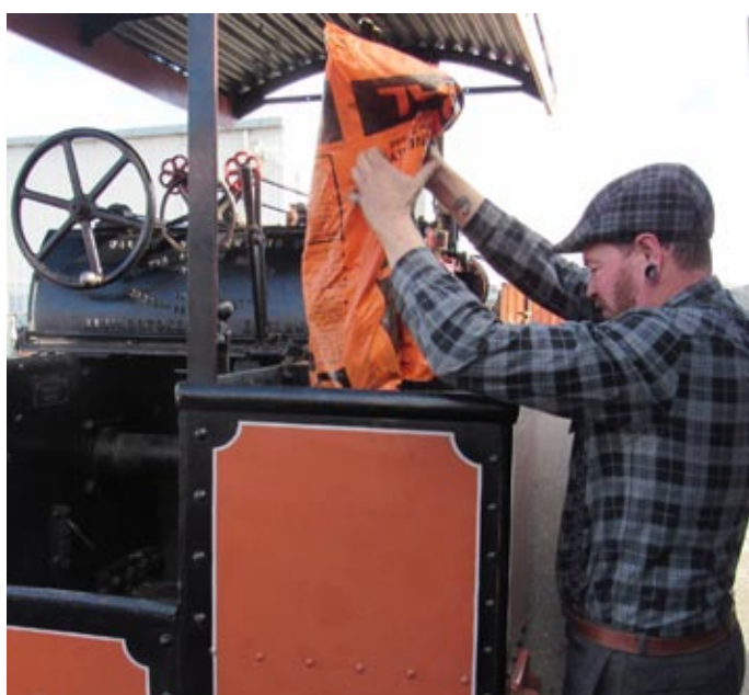
Andrew Holeyby fills the coal bunker on the MOTAT Wallis and Stevens steam roller.
