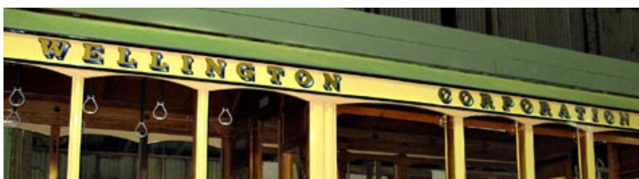
ABOVE: Computer generated vinyl signage on the cant rails.
