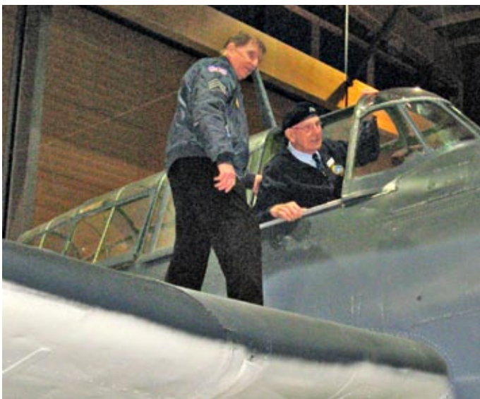
Peter Dilley, a former Fleet Air Arm engineer and Korean War veteran, at the controls of the Grumman Avenger, assisted by Henry Swan. The carrier based torpedo bomber has recently been restored to a standard where the folding wings work, and the bomb bay doors open and close, powered by an outside power source rather than through the aeroplane's own hydraulic system.
