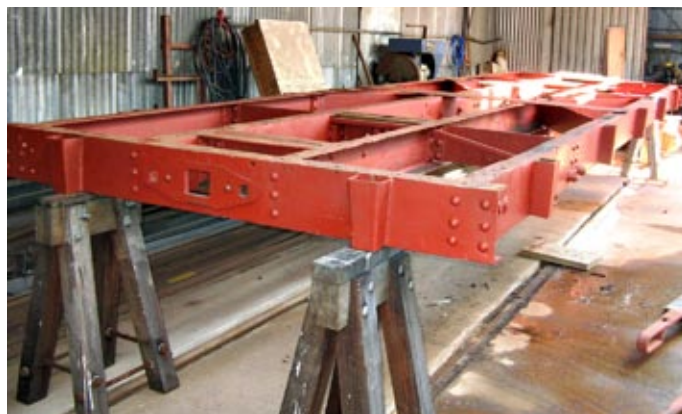
The chassis for the new runner wagon for crane 283 has received its coat of primer after metal work has been finished.
