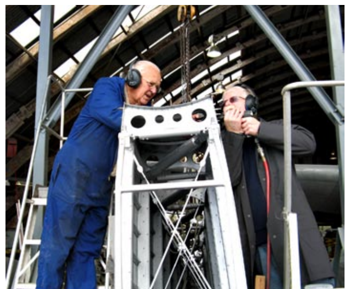
Working on the fin of the Short Sunderland flying boat are Norm McKelvie (left and Ron Wilson, as new metal is rivetted into place to replace corroded sections.
