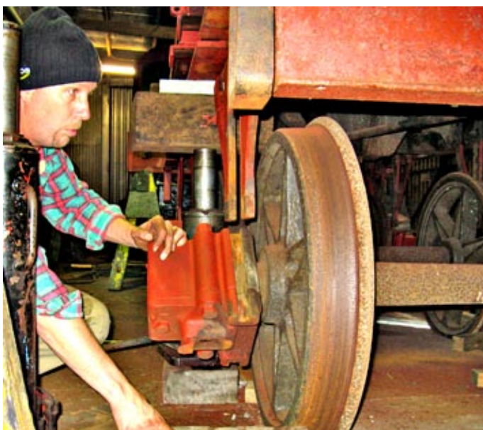
Pete Cairncross supervises the removal of the axles from crane 283. Evan James photo
