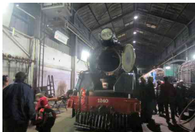
Lower photo, Mainline Steam's fully operational Ja 1240, with the smoke box door open, undergoing its annual boiler survey. Photos: T.Phillips
