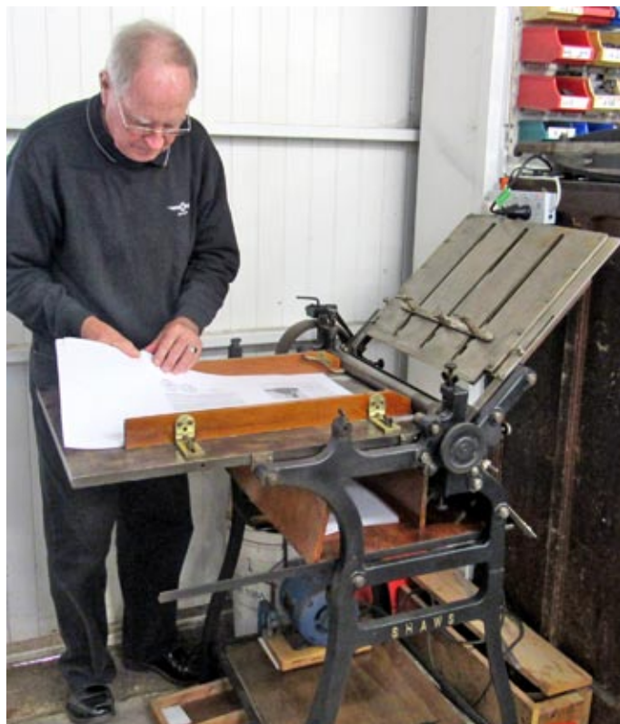
Print Section head Graham O’Keeffe hand feeding printed sheets of the Richard Pearce booklet into the recently restored Shaws Homley folder.
