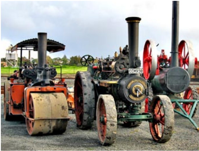
A line up of portable steam power, from left, a Wallis and Steevens steam roller, Fowler traction engine, and Marshall stationary steam engine.
