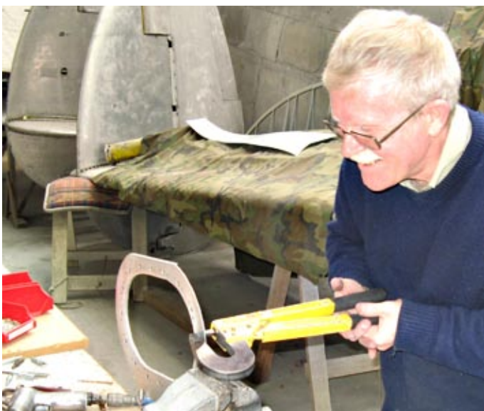
Ron Wilson uses a specialist tool for rivetting a new section for the Sunderland.
