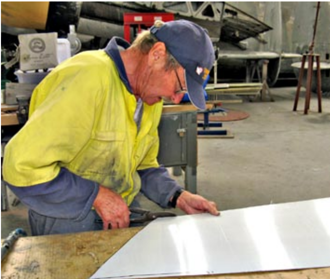
Hand skills come to the fore as Don Legg cuts aluminium sheet for a section of the Sunderland that is being replaced.
