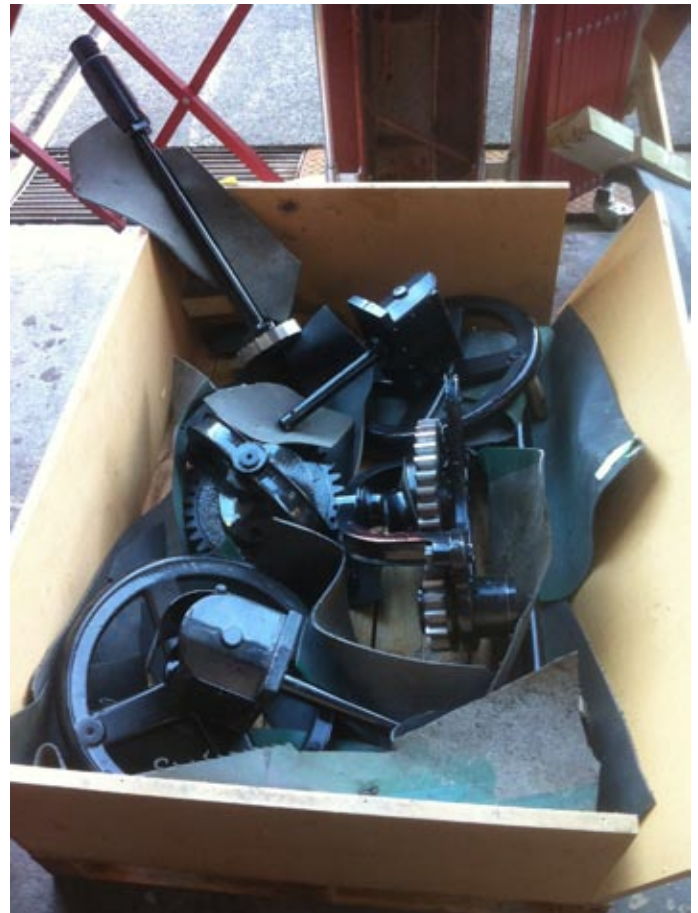
A box load of hand brake parts which arrived from the Tramway Heritage Trust of Ferrymead, Christchurch. They include a set of handbrake standards and underfloor chain snail gears, replicas of the originals, which were also manufactured in Christchurch, and the same as parts used on trams that have been restored in Christchurch.
