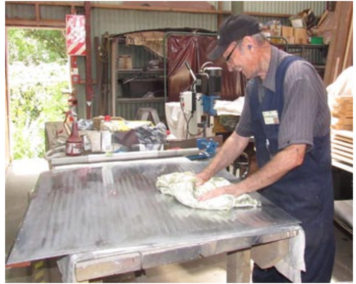
Tony Messenger gives a panel a final hand buff before it is ready for its trip to the anodisers. Once it is back from the anodisers the stiffeners can be attached to predrilled holes.
