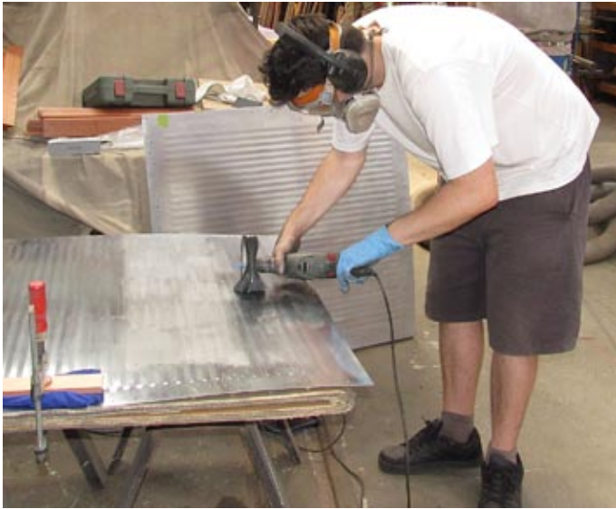
Joseph Dixon working away at an aluminium side/door panel with a buffing wheel as he works out the scratches and other imperfections.
