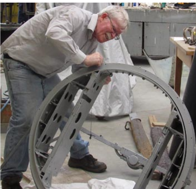
Meanwhile work on other aircraft in the collection continues as Ron Wilson works on a gun turret for the Short Sunderland flying boat
